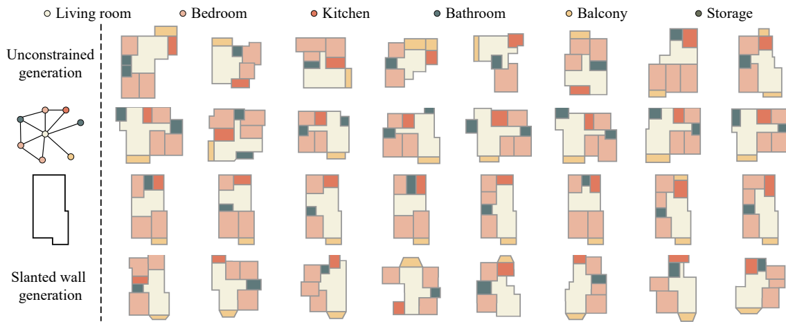
Figure 4: A gallery of vector floorplans generated using our framework. From top to bottom: unconstrained generation, topology-constrained generation, boundary-constrained generation, and unconstrained generation with slanted walls.
