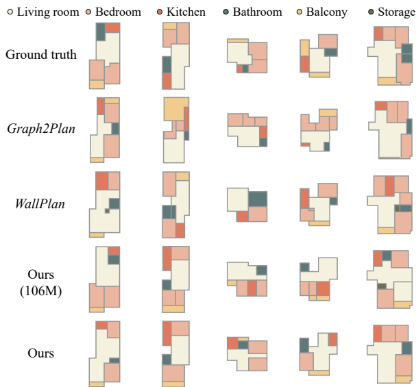
Figure 5: Comparison with the ground truth, Graph2Plan , and WallPlan on the boundary-constrained generation. Our method can produce more reasonable floorplans.
