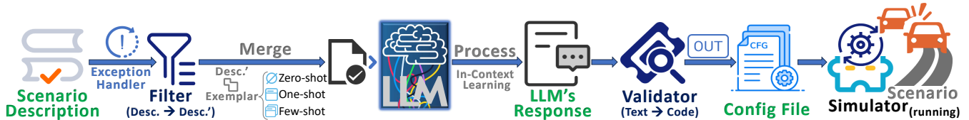
Figure 2: Architecture Overview. It begins with the user inputting a scenario description, which is managed by the Exception Handler to block adversarial or irrelevant inputs, ensuring the framework operates within scope and prevents downstream issues. The Filter processes the description, replacing simulator-incompatible terms with those aligned to the simulator’s documented APIs. The filtered description ( Desc. ) is combined with pre-constructed ICL exemplars, which can be zero-shot, one-shot, or few-shot in category, depending on the LLM’s familiarity with the simulator’s APIs and the complexity of the scenario. The LLM generates a response containing scenario configurations, often accompanied by explanations and comments. The Validator verifies each API call for compatibility, replacing unsupported terms with suitable alternatives (e.g., replacing “storm,” unsupported in CARLA, with “rain”) or ignoring them to prevent errors. This ensures all calls align with the simulator’s capabilities, enabling execution of the final configuration file. The simulator runs the scenario, with the final step depicting the interaction between the real world and the virtual environment, while data collection can take place either inside the simulator (as is the case in this study) or externally.
