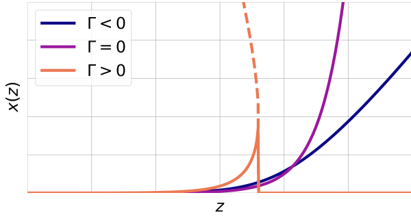
Figure 2: Sketch of x(z) for different values of \Gamma . The solution for \Gamma > 0 is double-valued below a critical z , as seen by the dotted lines. The bottom (solid) branch is of interest here.
