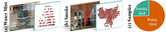
Figure 3: Random objects LiDAR Dataset (ROLiD). (a) and (b) are the data collection scheme and local point cloud visualization respectively. (c) represents the data used for the PCS-GAN network.
