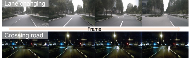
Figure 6: User-customized driving videos generated by DriveDreamer-2 . The top row depicts a scene where the ego car changes lanes, while the bottom row shows an unexpected pedestrian crossing the road at night.
