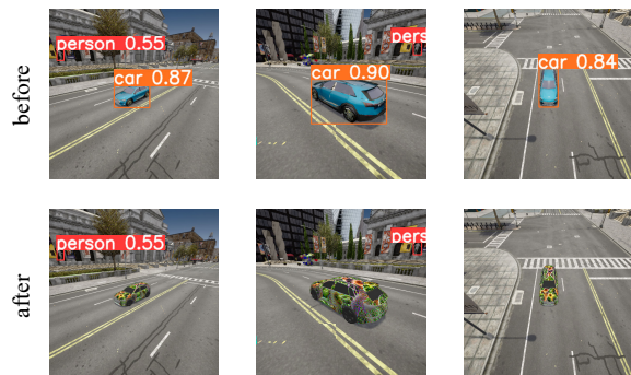
Figure 4: The detection result of the vehicle under different view angles before and after PhyCamo attack.
