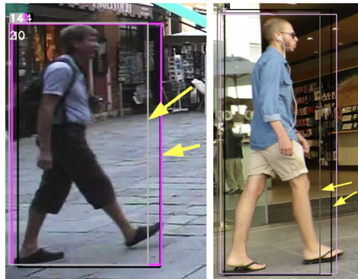
Figure 4: Visualization of Target Position Prediction. The true bounding box of the target in the previous frame is shown in gray, while the current frame’s true bounding box is in color. The predicted bounding box for the current frame, generated by the Position Predictor, is shown in black.
