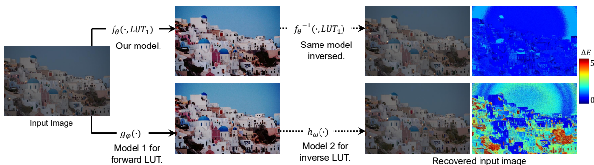
Figure 6: This figure compares the inversion accuracy of our modified invertible model versus a non-invertible architecture for estimating the forward and inverse pass through a single LUT. We use a deeper architecture ( D = 32 , hidden structure [16, 32, 16] ) to embed 32 LUTs, ensuring it remains bijective during training. We train a small architecture to estimate the LUT ( g_\psi ) and its inverse ( h_\omega ). Results are shown on an Adobe 5K dataset image processed by reconstructed LUTs, with \Delta E error maps computed per pixel against the ground truth image.
