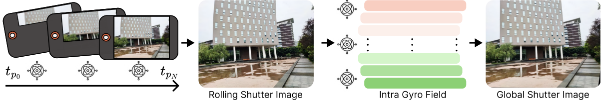
Figure 2: Rolling shutter image \mathbf{I}_{RS} , is introduced by high-frequency shake with a row-wise exposure CMOS camera. The gyroscope can accurately record these motions, which are then transformed into a motion field, \mathbf{G} \in \mathbb{R}^{2 \times H \times W} . This field is referred to as the Intra Gyro Field (IGF). With \mathbf{G} , we are able to correct \mathbf{I}_{RS} , resulting in a Global Shutter Image, \mathbf{I}_{GS} .
