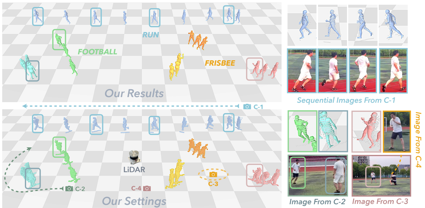
Figure 1: Visualization of our FreeCap in a real-time captured scenario. Our settings include a single LiDAR and four cameras. Camera-1 follows the running person, camera-2 surrounds two people playing soccer, camera-3 focuses on the main person playing frisbee and camera-4 captures three persons. We zoom in some cases to the right.
