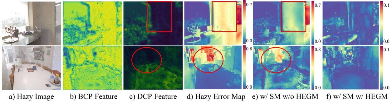
Figure 2: Visualization of the relationship between the spatial haze degradation(a)(d) and BCP(b) and DCP(c) in the deep feature domain. The error maps are differential values with reference, indicating haze distribution, shown in red boxes.
