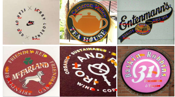
Figure 5: Qualitative results on the testing set of InverseText, Total-Text, SCUT-CTW1500 from left to right in the first line. The second line is the visualization of local grids predicted in MAAM for some challenging text instances. The color from light to deep indicates the decoding order.
