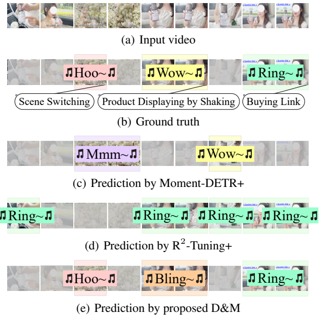
Figure 1: Illustration of video decoration with sound effects (VDSFX), aiming to automatically add proper SFX to key moments, which are also auto-detected, in a given E-commerce video. Moment-DETR+ and R^2 -Tuning+ are baselines we implement, by re-purposing Moment-DETR (Lei, Berg, and Bansal 2021) and R^2 -Tuning (Liu et al. 2024) for the new task, with their detected moments used for moment-to-SFX matching. Best viewed digitally.
