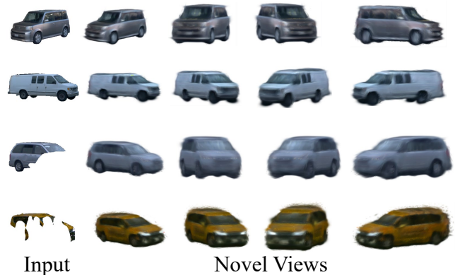
Figure 1: Driving scene data is often diverse, characterized by varying vehicle types, lighting conditions, and levels of occlusion. Our method aims to address the limitations of existing approaches by enabling the generation of unconstrained single-image to 3D vehicle models using only low-quality real-world data.
