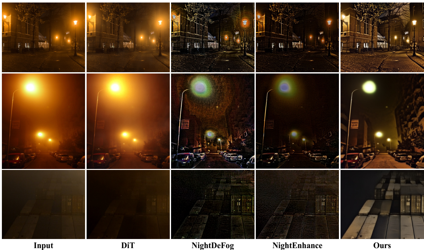
Figure 1: Qualitative results from NightEnhance’23 (Jin et al. 2023), NightDeFog’20 (Yan, Tan, and Dai 2020), DiT’23 (Peebles and Xie 2023) and our method, on the real-world dataset. Ours not only suppress glow but also reveal the detailed textures of the night scenes, including those under low light and strong glow.
