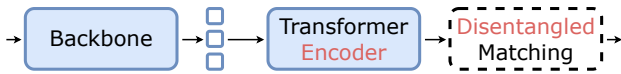
Figure 4: Comparison with existing transformed-based 3D object detection methods. We introduce encoder-only transformer architecture w/o positional encoding for queries or attention layers. This allows us to change unstable Hungarian matching for a simpler disentangled scheme.
