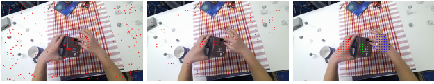
Figure 3: Query location visualization: (a) Left : query locations of H2OTR (Cho et al. 2023), employing 300 queries. Notably, a substantial amount of queries are distributed in backgrounds. (b) Middle : Our hand-object query locations w/o Query division block. Due to feature similarities between two hands, a considerable number of queries concentrate on the left hand than the right hand, which reduces the accuracy of the right hand. (c) Right : Our hand-object query locations. Queries for left and right hands are highlighted in red and blue, respectively. Queries for objects are denoted as green. The query proposal loss ensures that each query concentrates on its specific region of interest.
