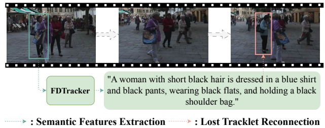
Figure 1: FDTracker provide accurate verbal descriptions of personal attributes. Thus, when a person disappears for a period of time and reappears, it can be reconnected to the original tracklet based on the appearance description.
