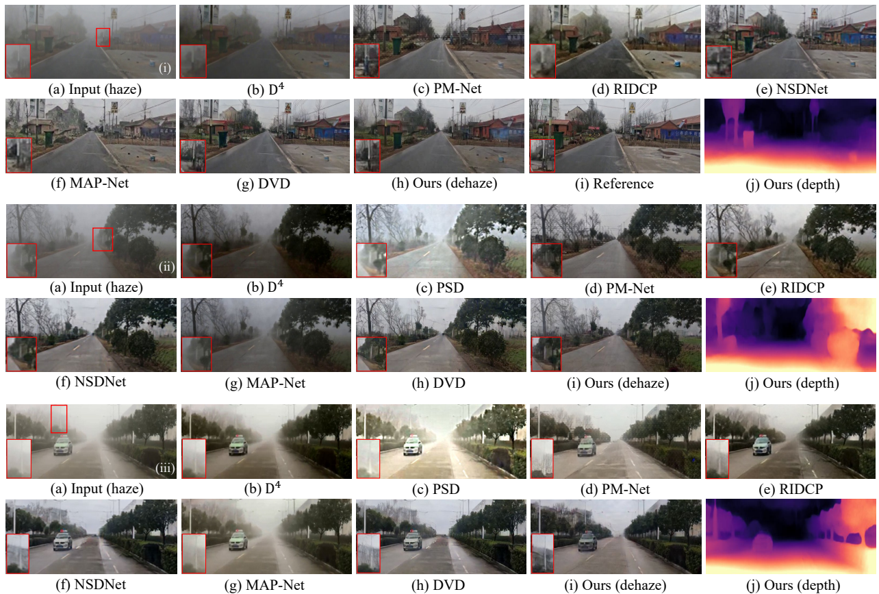
Figure 3: Comparisons of video dehazing performance across (i) GoProHazy, (ii) DrivingHazy, and (iii) InternetHazy. Our method effectively removes haze and accurately estimates depth. The red box highlights a zoomed-in region for clearer comparison.
