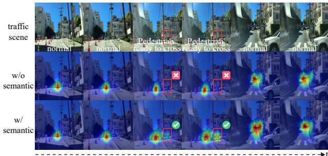
Figure 7: Visualize the driver’s attention under the semantic information of a pedestrian ready to cross the road.
