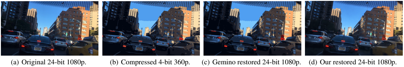
Figure 2: Visualization of a frame in the NeVS pipeline: (a) original 24-bit 1080p, (b) 4-bit 360p by encoder’s resolution-color compression, (c) restored 24-bit 1080p by Gemino’s decoder, and (d) restored 24-bit 1080p by our DeNC’s decoder with much higher perceptual quality, e.g. , see the sky color transition and car license number. Best viewed in color and zoomed-in.
