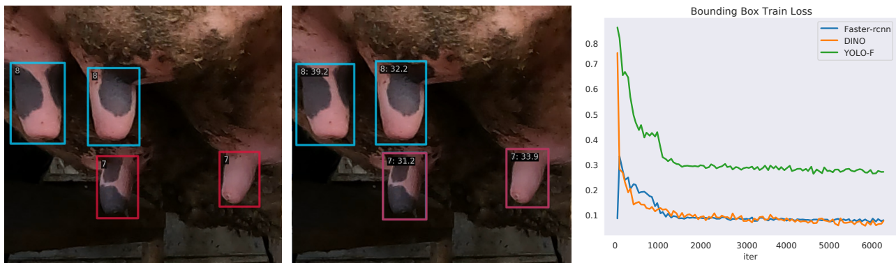
Figure 1: (Left) Using LabelMe to draw bounding boxes and precisely annotate cow teats with the scores provided by the expert veterinarian. (Middle) ML predictions of each teat shape’s score. (Right) A plot of the bounding box train loss vs. training iterations
