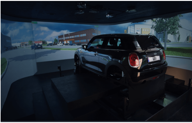
Figure 2: High-fidelity traffic simulator developed at Way AS. A real car is mounted on the motion platform in the center. Surrounding the car is a projection screen wall with six different view channels projected at the driver's front.
