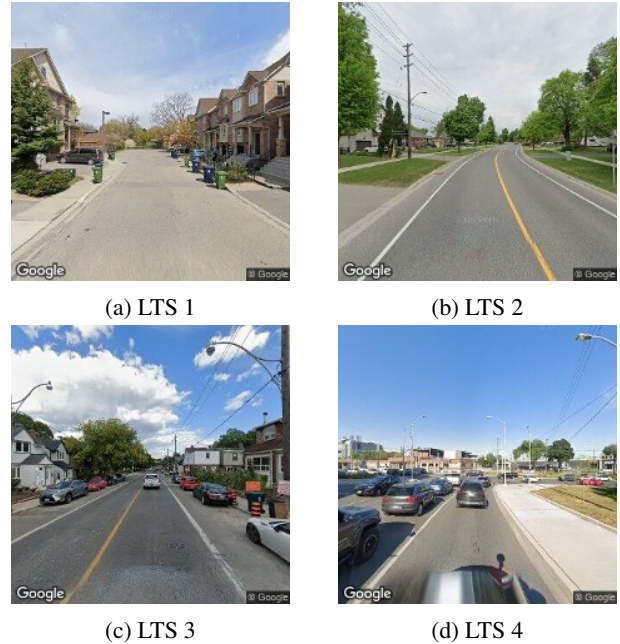
Figure 1: Example images with the four LTS labels: LTS 1 roads are safe for all cyclists including children, LTS 2 roads are for most adults, LTS 3 and LTS 4 are for “enthusied and confident” and “strong and fearless” cyclists, respectively.
