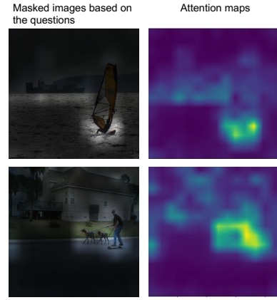
Figure 5: The attention mechanism identifies the important regions that are relevant to answering the given question. These attention maps were generated by computing the weight matrix from the attention mechanism. The top images are associated with a question asking about the color of the sail, and the sail is highlighted. The bottom images are associated with a question asking about the number of dogs the man is walking, and the dogs are highlighted.
