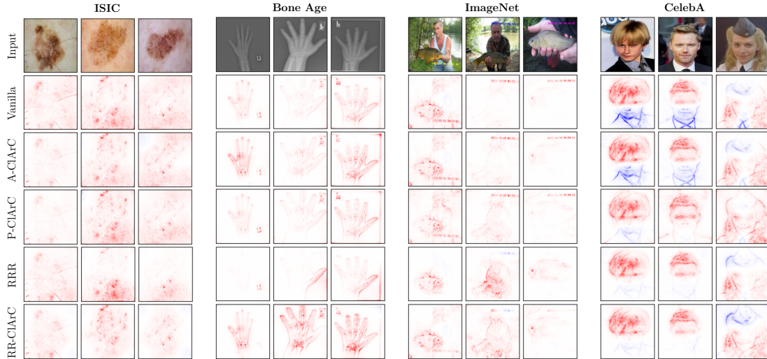
Figure 4: Effect of model correction on explanation heatmaps for the VGG-16 model on all datasets. Whereas RRR successfully decreases the relevance on localized biases (ImageNet and CelebA), RRR tends to fail on unlocalized artifacts (ISIC, Bone Age), with the model’s attention focusing on arbitrary features. Overall, RR-CIArC reduces bias attention most reliably.
