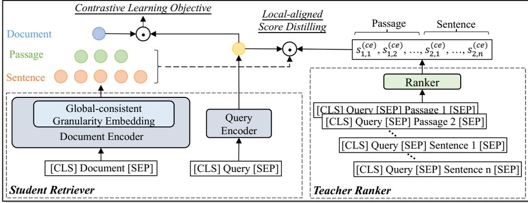
Figure 2: An overview of our fine-grained distillation (FGD) for long-document retrieval. FGD uses a global-consistent granularity embedding method to produce representations for different granularity in a document. Then, FGD applies a local-aligned score distilling strategy to learn from a cross-encoder teacher at each granularity level. Finally, a hierarchical hard negative mining provides negative samples across granularity.
