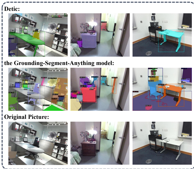
Figure 2: Bounding boxes generated by the Grounded-Segment-Anything model and Detic Original pictures are selected from the SUN RGB-D dataset.
