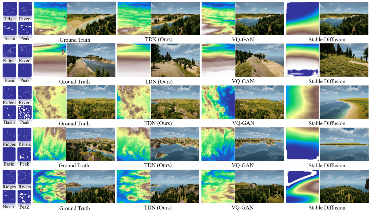
Figure 3: Comparisons between various terrain generation methods with user input sketches, height map and rendered view.
