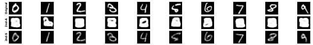
Figure 11: Reconstructed images of the MNIST dataset for SIM with link function (20) and Rayleigh sensing vectors. The number of measurements m = 400 .
