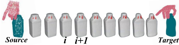
Figure 5: Grasp transfer from one instance to another instance of the same category.
