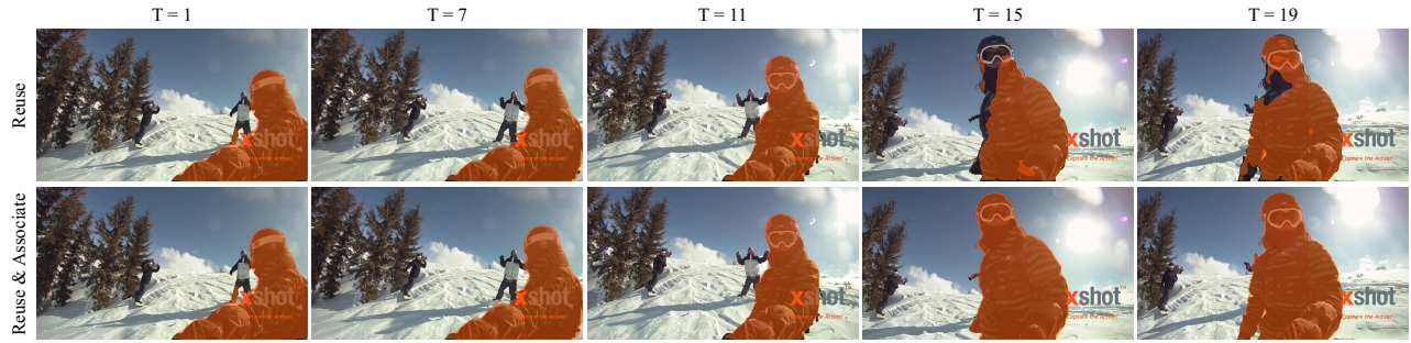
Figure 2: Reusing kernels for tracking. We train MobileInst for single-frame instance segmentation on YouTube-VIS 2019, and then apply MobileInst to infer the per-frame segmentation and track objects via reusing mask kernels. The upper row: We adopt the predicted mask kernel in T = 1 frame to obtain the segmentation results in the video sequence. In a short time, the reused mask kernels provide accurate segmentation and tracking results. The bottom row: We divide the videos into K -frame clips and reuse the mask kernels of every first frame. In addition, we adopt simple yet effective cosine similarity to associate the kernels in consecutive clips ( K is set to 3). Reusing kernels with association performs well and is efficient.
