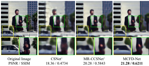
Figure 6: The reconstruction results at an extremely low (1.5625%) sampling rate show that competitive methods produce distorted or erroneous results in the restoration of hand and car window contours, while our method still achieves the highest quality.
