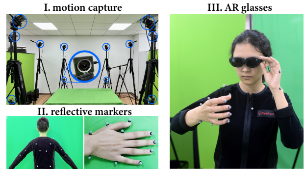
Figure 2: Illustration of recording setup (MoCap + AR glasses).
