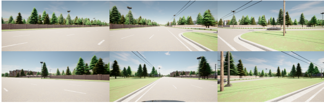
Figure 3: A scenario where a vehicle is going to merge from the entrance ramp. From top left to right bottom are images captured from FrontLeft, Front, FrontRight, BackLeft, Back, and BackRight cameras. The vehicle is invisible in the Front view but can be seen in the FrontRight view.
