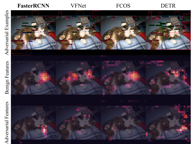
Figure 1: Adversarial examples crafted on FasterRCNN by our method effectively suppress the significant features and amplify the vicinal ones in both surrogate and target models. High-brightness areas correspond to high-value features.
