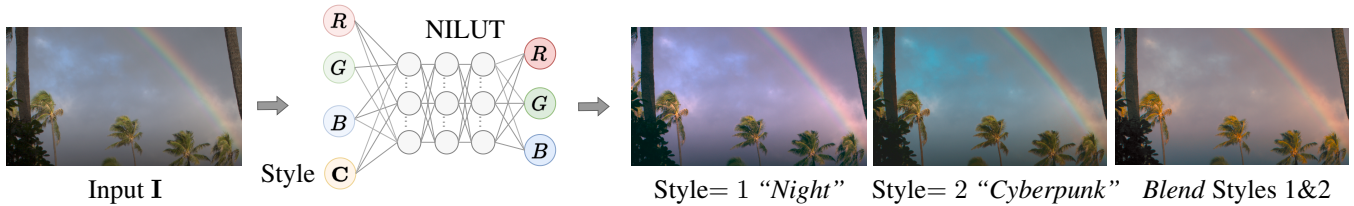
Figure 2: NILUTs encode multiple 3D LUTs in a single representation with the ability to blend between “styles” implicitly.
