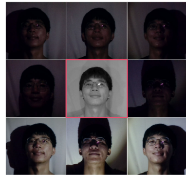
Figure 1: Comparison of VIS and NIR facial images under extreme lighting. The red frame in the center of the figure is NIR images. Even under low lighting or complete darkness, the geometric and texture details of volunteers in NIR images are still very well preserved.
