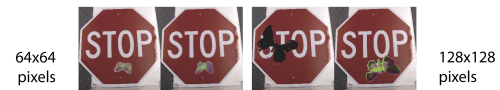
Figure 2: By placing a moth-like patch on a ‘STOP’ sign, we can make autonomous driving cars misrecognize the sign as ‘Speed Limit 80’ (Yakura et al. 2020).
