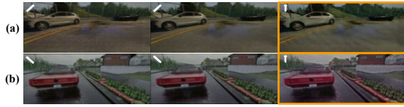
Figure 6: Test images generated by FtGAN for CARLA-CNN. We observe (a) the center line wear-out and road texture changes, and (b) the color tone changes.
