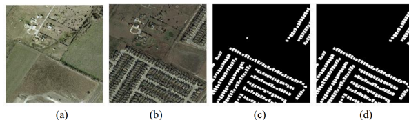
Figure 1: Result of our model for change detection in the LEVIR-CD dataset. (a) and (b) input remote sensing images, (c) ground truth, and (d) prediction result of our model.
