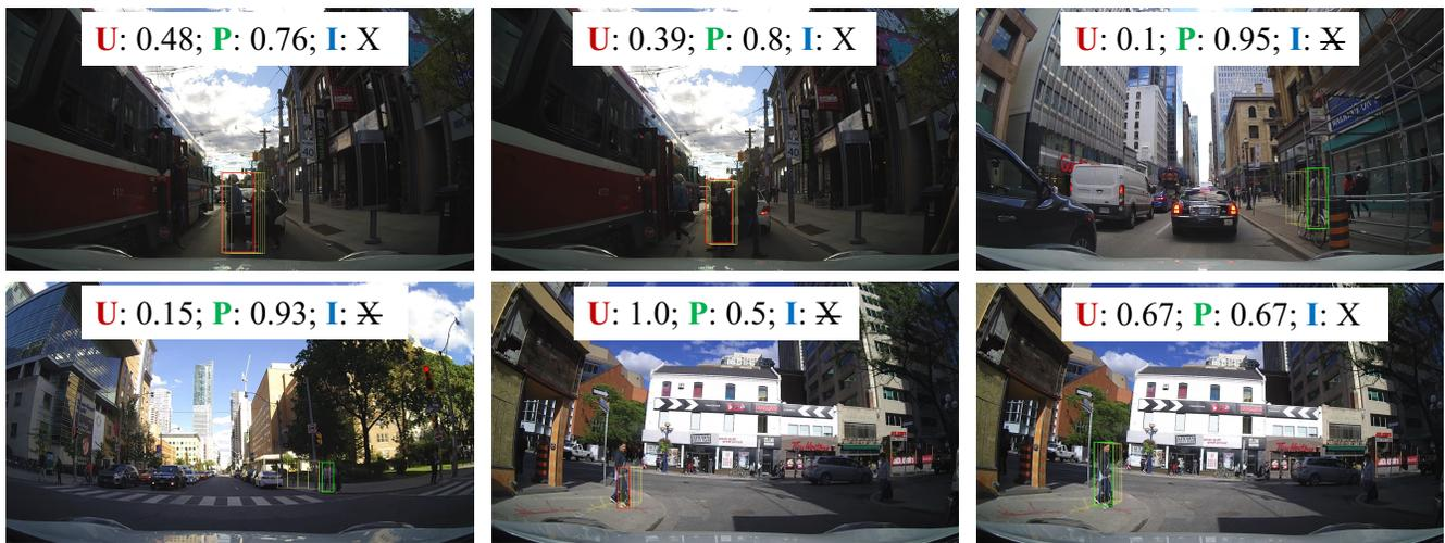
Figure 4: Case study on PIE dataset, where U denotes the uncertainty, P means probability and I represents the decision ( $X$  is crossing, while the crossed  $X$  is not crossing). The red bounding boxes indicate the cases where our model predicts wrongly, while the green bounding boxes are the correct cases. The yellow bounding boxes are those in the previous 3 frames.
