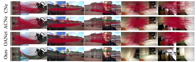
Figure 6: Visualizations of camera pose estimation. Red/Green indicates incorrect/correct correspondences.
