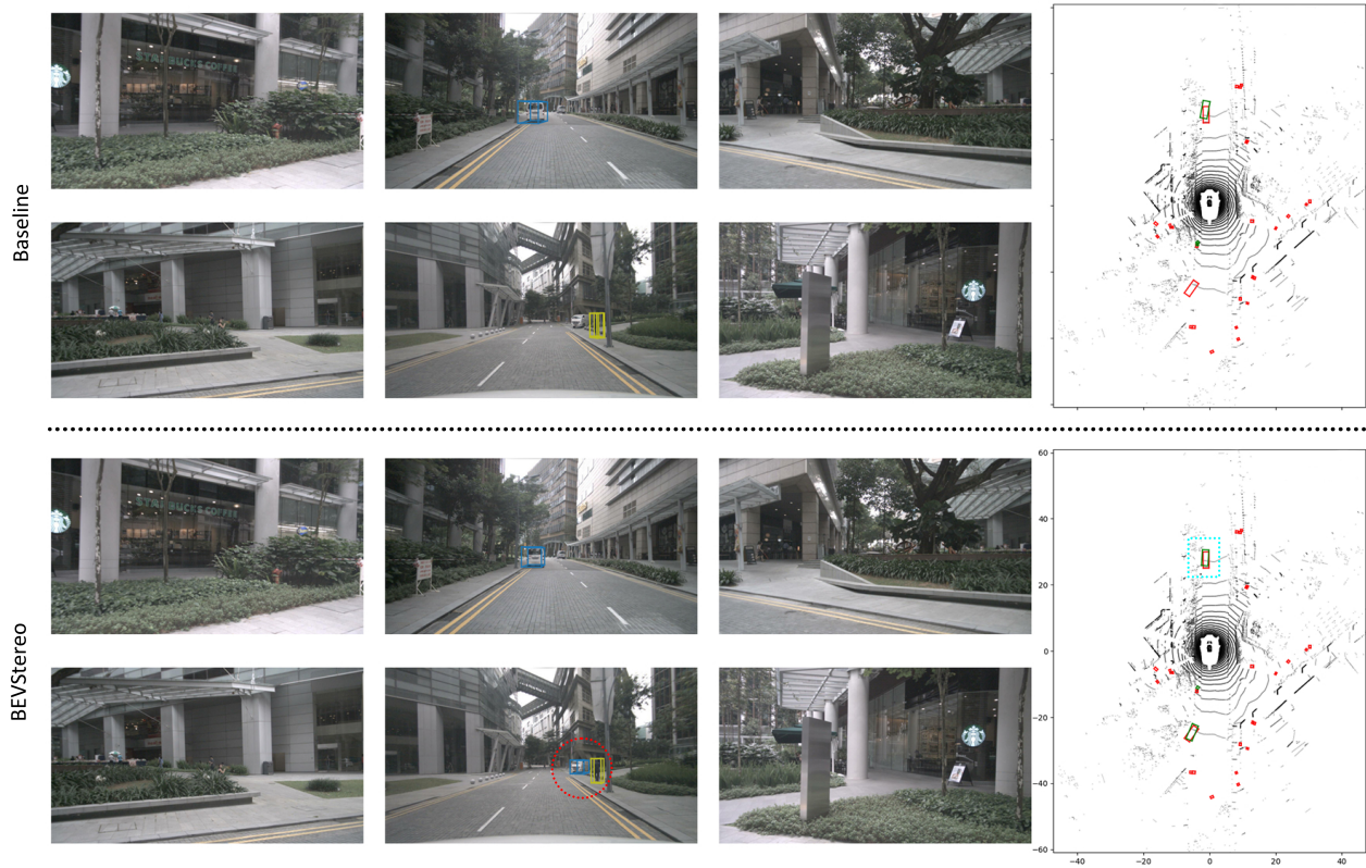
Figure 6: Visualization of detection results. The blue dotted rectangle designates the object recognized by our approach is more accurate on localization, while the red dotted circle designates the object detected by BEVStereo but missed by the baseline.
