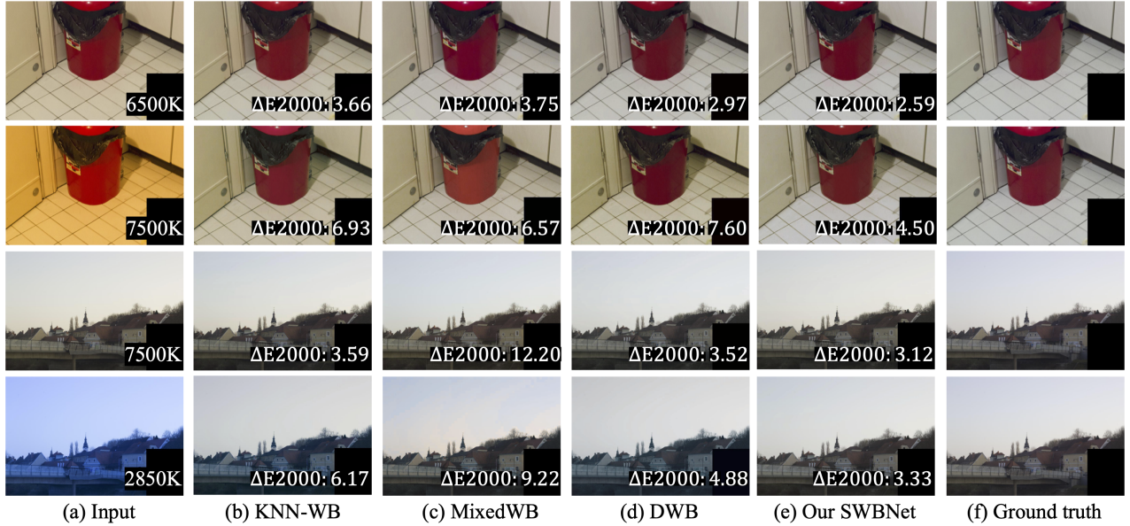
Figure 8: Qualitative comparison for WB stability. The \Delta E_{2000} value is marked in the bottom right of the image.
