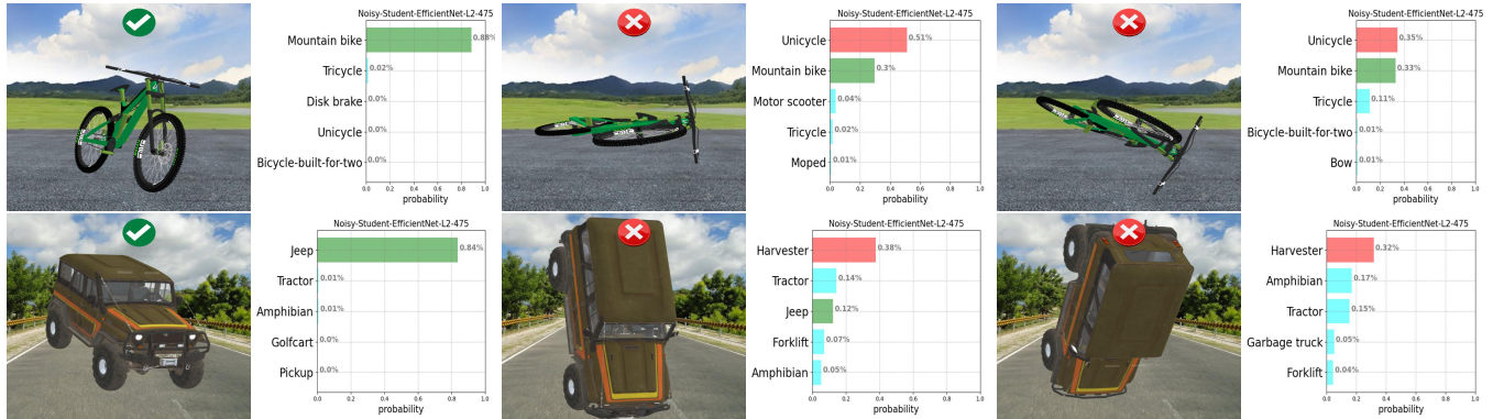
Figure 3: Selected failures of Noisy Student EfficientNet-L2—the best-performing network of our collection—on ObjectPose. Left column: Objects presented upright and top-5 predictions from the network (as measured by the softmax layer activations). Other columns: Objects presented in incorrectly classified poses and top-5 predictions from the network. Some of these errors reveal a brittleness compared to the human visual system (e.g., a tank at 90^\circ is confused with a shield).
