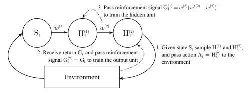
Figure 1: Illustration of a network with two units trained by Weight Maximization. See text for explanation.
