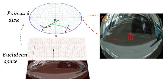
Figure 1: Learning deformable kernels in hyperbolic space for adapting CNNs to large FoV (fisheye) images. Image and input feature maps are represented on a graph and mapped to the Poincaré disk for learning positions in a  $(k \times k)$  receptive field  $K_x$  at every spatial location  $x$ .
