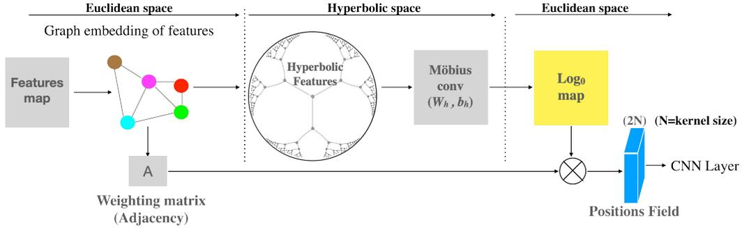
Figure 3: FisheyeHDK convolution layer. HDK network is one hyperbolic convolution layer predicting the positions in a deformable kernel of size  $(k \times k)$  for each point of the spatial support. Conventional (Euclidean) convolution is applied between the weights sampled at predicted positions and input feature map.
