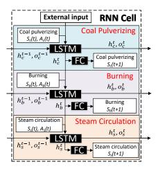
Figure 2: Design of the combustion process simulator
