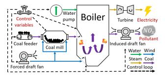
Figure 1: Illustration of operation mechanisms of a TPGU
