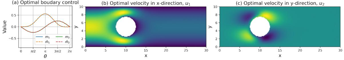
Figure 3: Illustration of the boundary control of the Stokes equation. (a) The control inputs  $m_1$  and  $m_2$  which correspond to the Dirichlet boundary values on the circle. The solid lines indicate the optimal control obtained by our method, and the dashed lines are the reconstructed control. (b), (c) The corresponding velocity fields  $u_1$  and  $u_2$  that minimize the drag energy.
